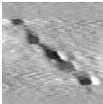
FIGURE 2 Image of a modified area of the silicon surface under the positive voltage (morphology and profile). The modification voltage: U_{\text{mod}} = 3.7\text{--}5.3\text{ V} , the visualization voltage: U_{\text{vis}} = 3.26\text{ V} . The size of modified areas – 0.5 \times 0.5\text{ }\mu\text{m} , depth – 6\text{--}15\text{ nm} .
